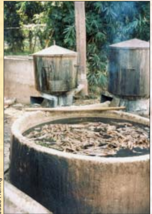
First soaked in water, the bark is then boiled in cauldrons to soften the fiber.
