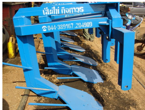
Photo 2: Cassava Digger for Big Tractor (>60 HP) Produced by Lert Engineering, Chonburi Province
