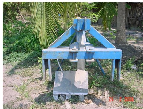
Photo 2: Cassava Digger for Big Tractor (>60 HP) Produced by Lert Engineering, Chonburi Province
